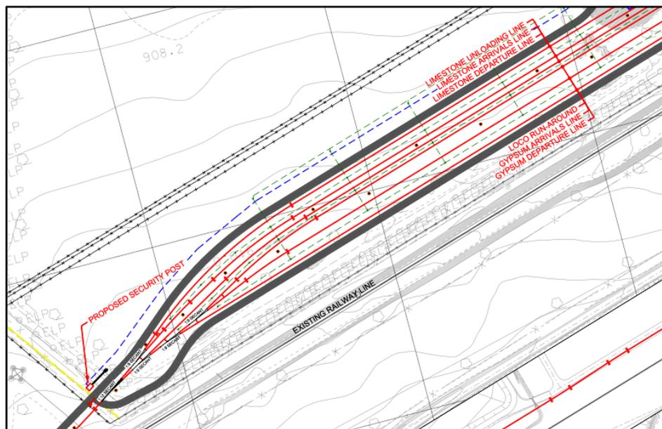
**Figure 6-8: Proposed alignment and layout of the rail infrastructure**
