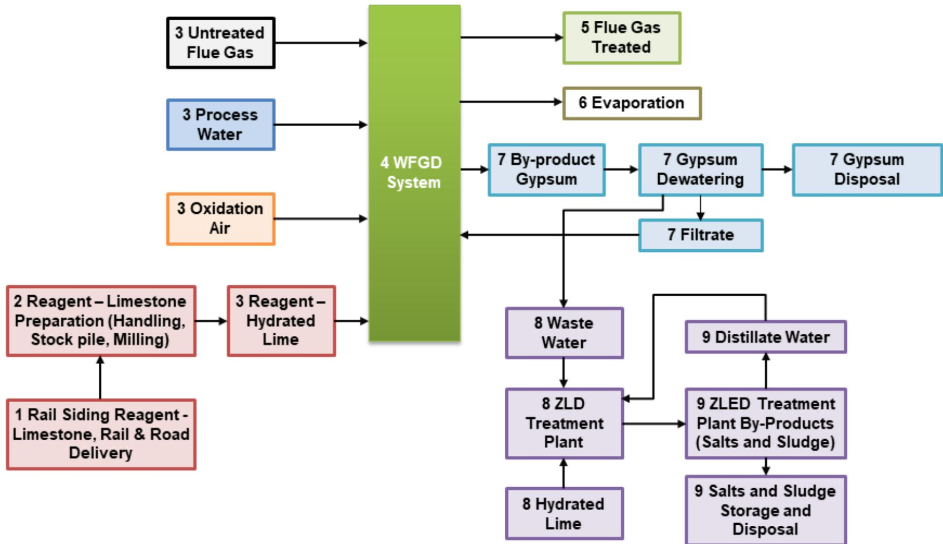
Figure 6-6: Basic Flow Diagram of Medupi FGD Process
