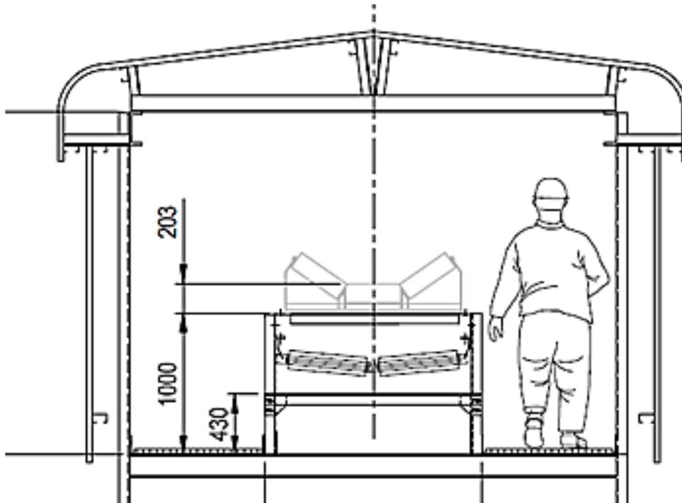
**Figure 6-18: Conveyor belt typical cross section**
