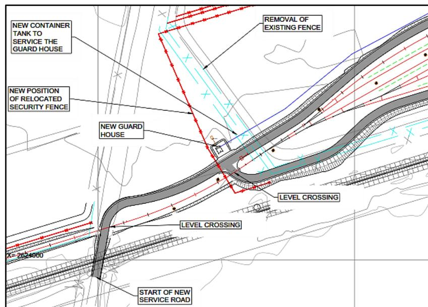
**Figure 6-11: Proposed security office and relocated security fence**
