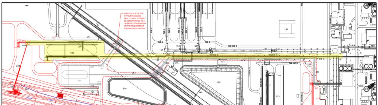
**Figure 6-17: Proposed limestone handling infrastructure (Block 2) shaded in yellow**
